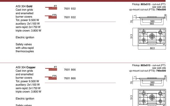
Safety valves with ultra-rapid thermocouples
