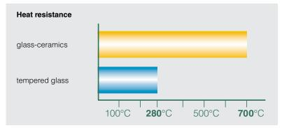
The top of the Ceramik hobs is made of glass-ceramics and not of tempered glass, like most of the gas hobs of this type. This ensures a greater resistance to high temperatures, thus preventing any possibility of glass explosion.
